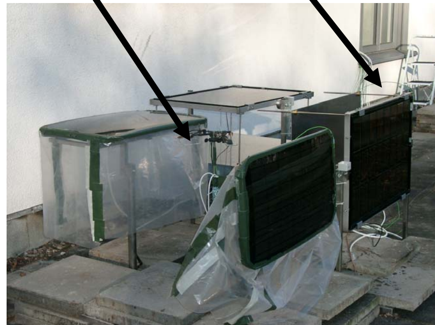
Testing facility on the institut's roof: Cells in vertical and horizontal orientation
